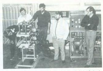
Collaboration between the School of Forestry and the Mechanical Engineering Department has resulted in the completion of the compression rolling machine, shown here, which will be used in a research project of considerable interest to the timber industry.
